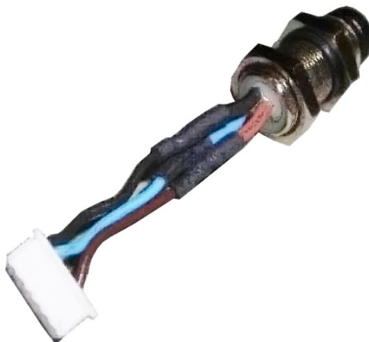
Figure 5-5— Threshold Relay Pico-to-Molex wire harness
